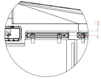
3b. Insert  $\frac{1}{4}$ -20 x  $\frac{1}{8}$  button head cap screws in the track and through the blind.
