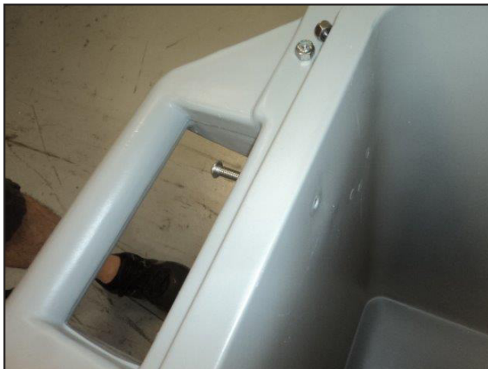
(6) Reinstall new bottom bolt
