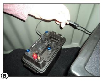
(11) Plug in 5-12 volt power supply (not included) using USB-C plug connection
