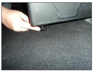
(6) Level fan box by screwing feet in or out
