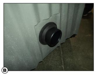
(5) Place fan box outlet tube through grommet hole inside blind
