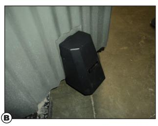
(7) Slide exhaust snorkel over outlet tube until it seals on tapered grommet
