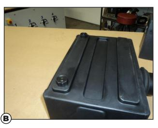
(3) Install both leveling feet in bottom of fan box
